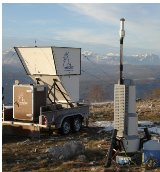
Figure 1: The measurement site Maligrad with the SODAR (left) and the ZephIR LIDAR (right).
